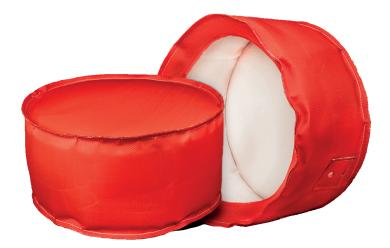
Fire hoods are a requirement for all in-ceiling speakers that are installed in or adjacent to habitable rooms or within a location of access or escape. Cutting large holes in ceilings for in ceiling speakers destroys the fire barrier and under UK Law the installer is responsible for maintaining that barrier when installing any equipment.
